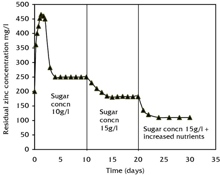
Figure 5. Change in residual zinc concentration with time at different sugar concentrations with proportional increase of nutrients
