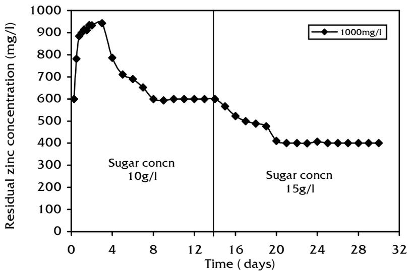
Figure 6. Change in residual zinc concentration with time at 1000mg/l of zinc concentration
