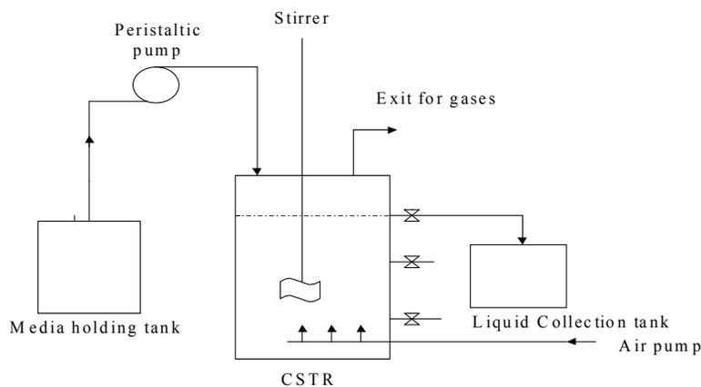
Figure 1. Schematic diagram of the reactor assembly
