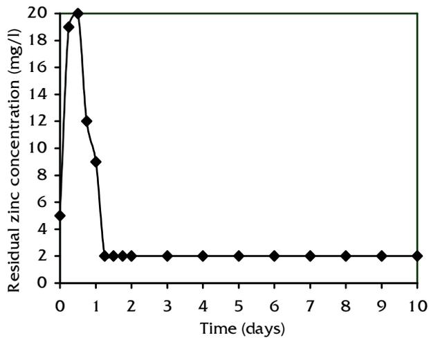
Figure 7. Change in residual zinc concentration with time in effluent
