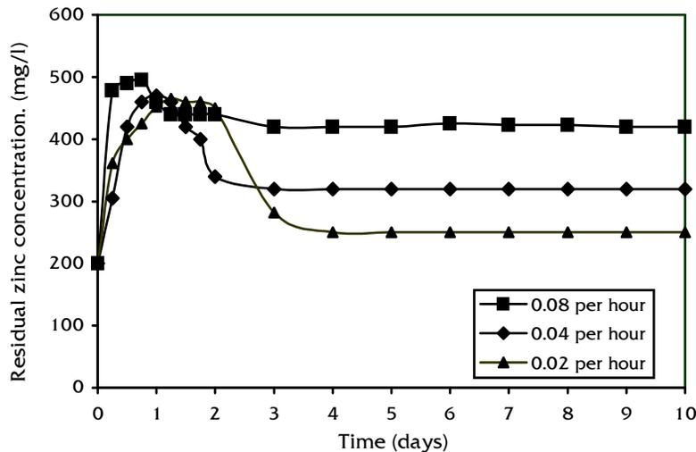
Figure 3. Change in residual zinc concentration with time at different dilution rates
