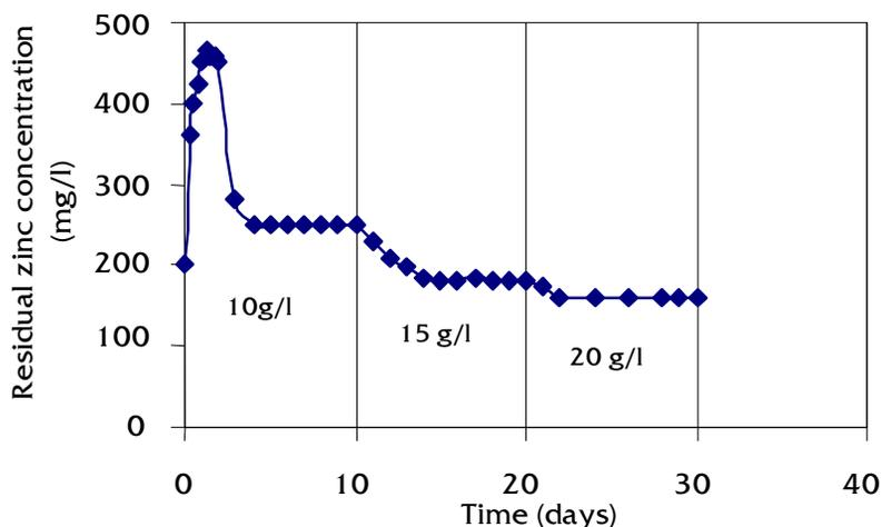
Figure 4. Change of residual zinc concentration with time at different sugar concentrations
