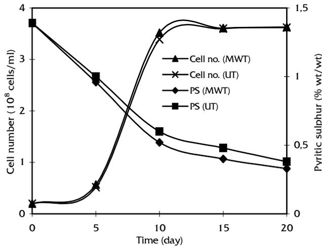
Figure 1. Change in pyritic sulphur and cell number during biodesulphurization of microwave treated (MWT) and untreated (UT) coal
