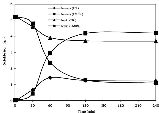
Figure 3. Change in ferric and ferrous iron concentrations during pretreatment of coal with *Thiobacillus ferrooxidans* bacterial liquor (TBL) and membrane filtered bacterial liquor (TMFBL)
