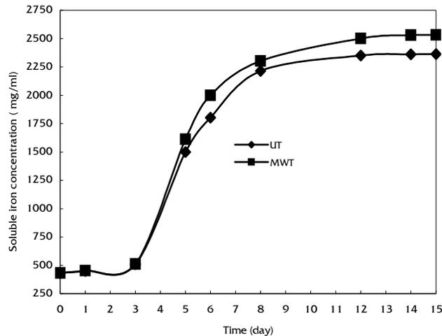
Figure 2. Change in soluble iron concentrations during biodesulphurization of microwave treated (MWT) and untreated (UT) coal
